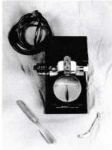
Figure 3—Liquid Limit Device with Soil Sample in Place
